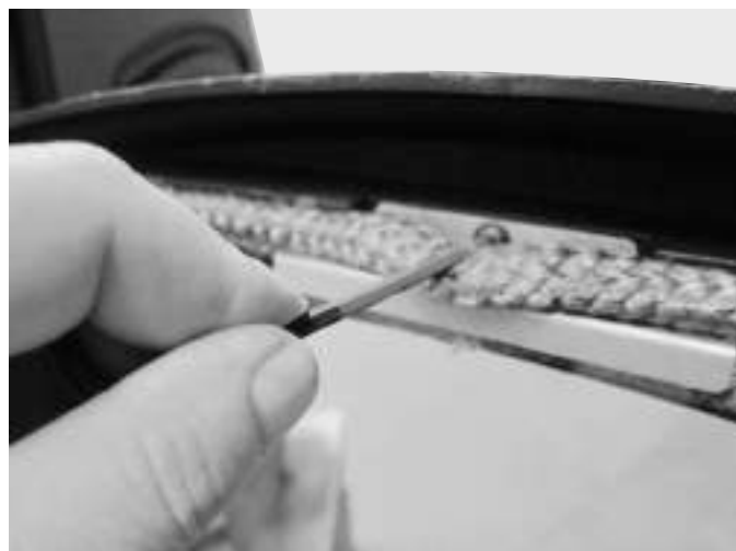
Figure 20. Loosen the glass clips.
