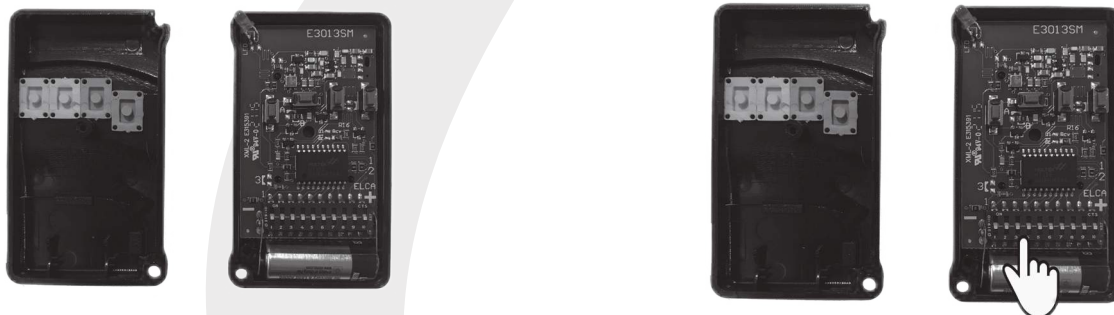
Change one of these 10 dip-switches
