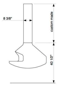
Diagram shows clearance to non-combustible flooring. For combustible flooring, please refer to P.7 diagram.
