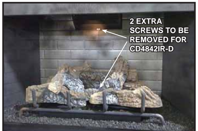
Figure 3.7 CD4842IR-D Extra Metal Refractory Screws
