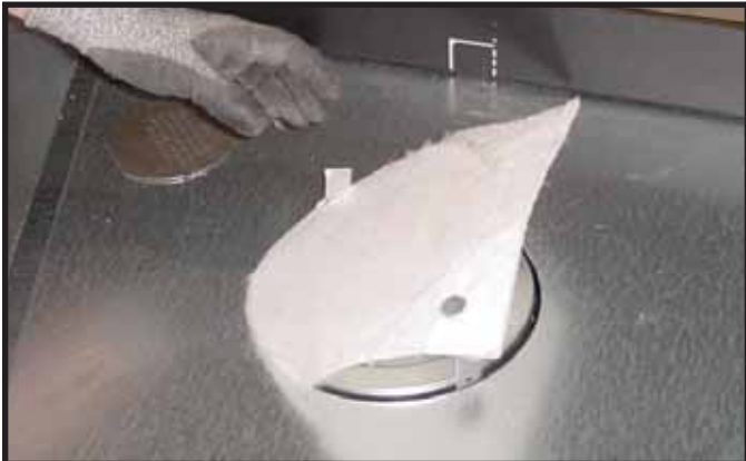
Figure 9.2 Remove the white gasket material covering the seal cap.
