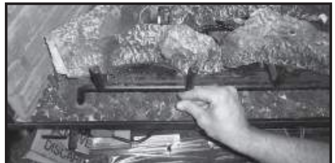
Figure 14.4 Placement of Vermiculite
