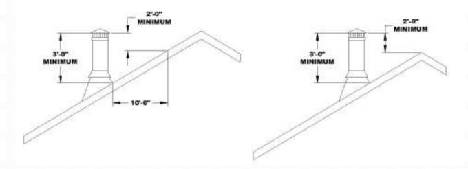
Figure 8 - Chimney Height Requirements
