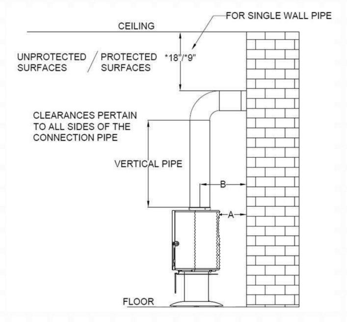
**Figure 5 Chimney Connector Clearances**
