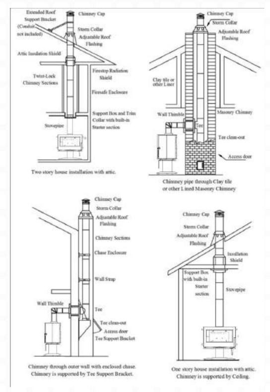
Figure 9 - Typical Chimney Configurations
