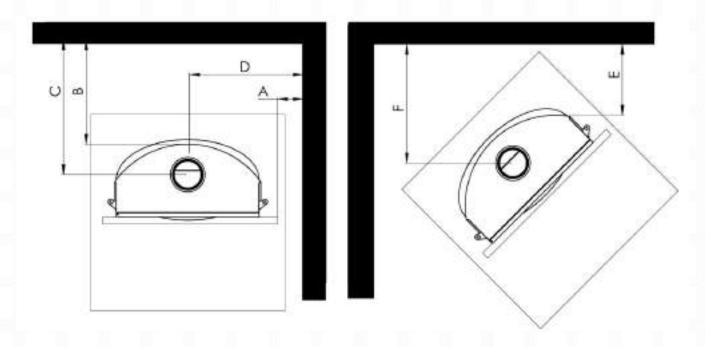
Figure 4 – Clearance to Combustibles
