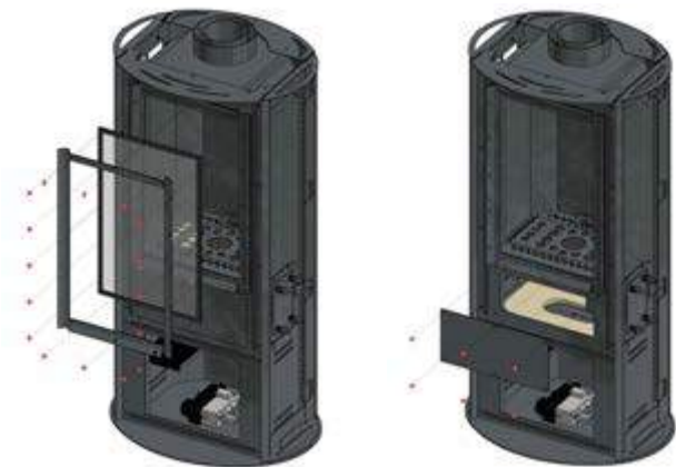
Figure. 11. Disassembly of the inner glass and revision of the stove
