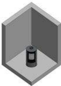
Figure 3. Location of the gas stove from the flammable housing components.
