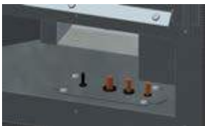
Figure 7. The way of routing out and sealing the capillary cable, the magneto wire, the tube of the main burner and the tube of the control burner
