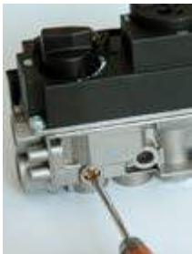
Figure 15. Adjusting method for the minimum flame height of the main burner
