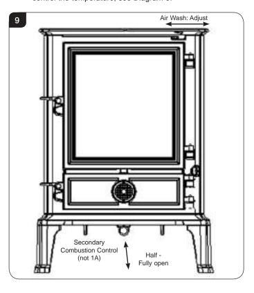
Leave the **Secondary Combustion control** open. The position will vary between half and fully open depending on the flue draught.
