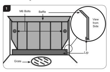
Lift the baffle clear of the lip and pull the bottom toward the front of the appliance so the baffle lies flat on the grate, see Diagram 2.
