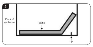
Using a combination of vertical and horizontal twisting lever the baffle loose and pull forward to remove through the front of the appliance, see Diagram 3.
