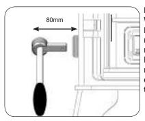
Note: When installing a Multi-fuel appliance a minimum gap of 80mm must be left on the Left Hand Side so that the riddling tool can be comfortably engaged in the socket.
