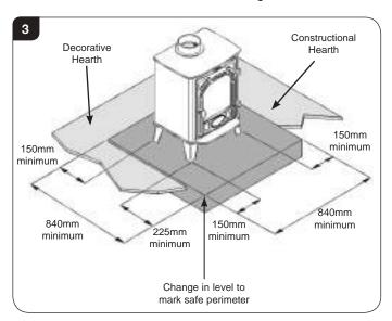
3.2 If this appliance is installed in an elevated setting it is recommended to increase the 225mm hearth depth to safely contain any falling logs or embers. The higher the appliance is installed the deeper the hearth should be to avoid scorched floor coverings.
