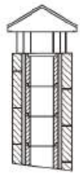
(2) Traditional chimney. The proper exit section must be, at least, two times the interior section of the chimney, the best is 2,5 times.
